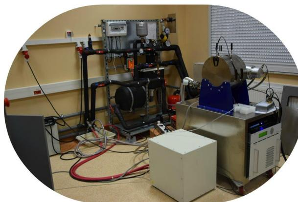
Spectrometer NMR with electromagnes 3 T (Tesle)
