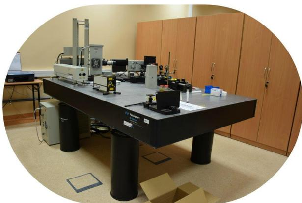
Spectrometer photoacoustic with laser and OPO
